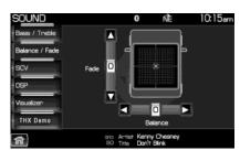
**SCV** (Speed compensated volume): With this feature on, the radio volume changes automatically with vehicle speed to compensate for road and wind noise. Select a level of compensation between 1 and 7 by pressing the corresponding button.
